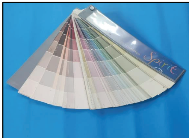
Figure 1 : The color chart used for determining color changes (Elite Paint & Chemical Industries Ltd., 1050 collection of spirit color chart).
